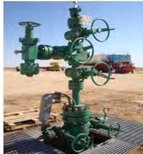
Typical Oil Well head
